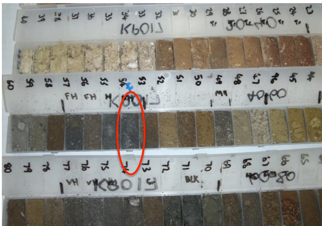
Koppio drillhole KP017 chip tray highlighting the 53-54m interval at 42.8% TGC
